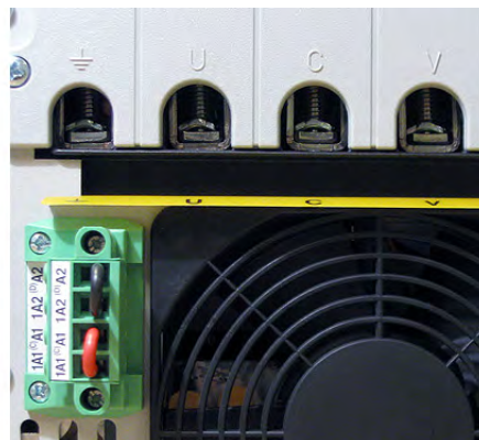
Shown with terminals jumpered for internal armature voltage feedback.
