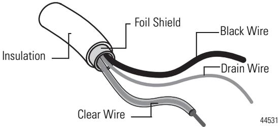
**IMPORTANT** Do not ground the drain wire and foil shield at both ends of the cable.
